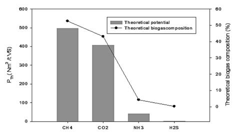
Figure 3. Theoretical potential and biogas composition of coffee waste using Buswell equation
